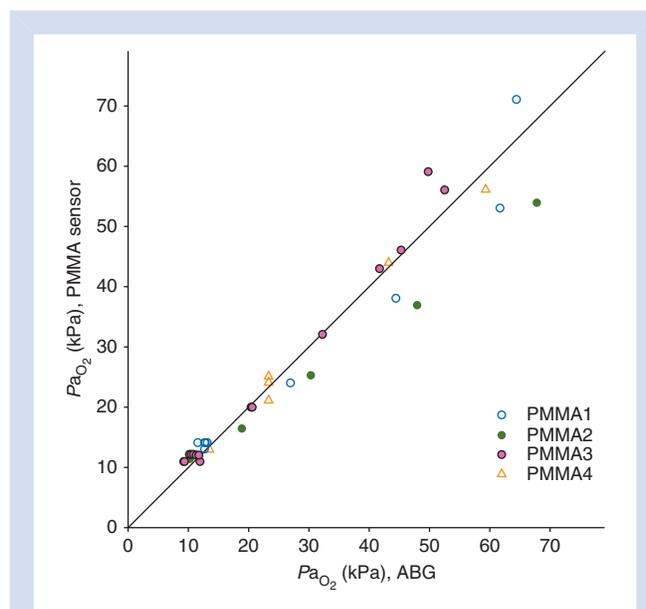
**Fig 2** PMMA sensor  $P_{aO_2}$  results (average value for 2 s) plotted against standard ABG analysis results ( $n=39$ ). Sensors coded PMMA1, PMMA2, and PMMA3 were used in the ovine models; sensor PMMA4 was used in the porcine model. The identity line illustrates the degree of agreement between ABG analysis and the PMMA sensor.
