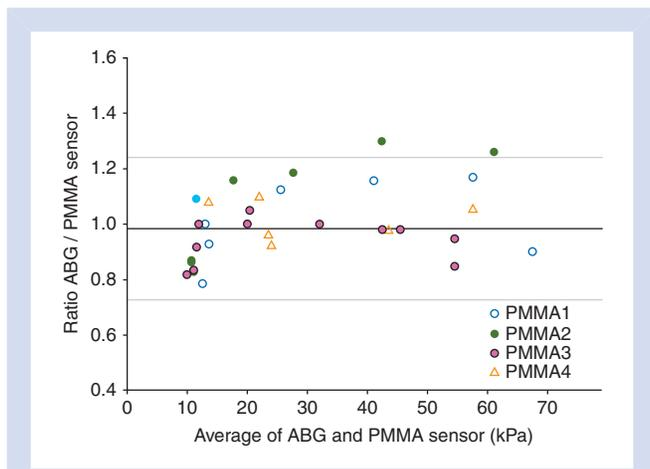
**Fig 3**  $Pa_{O_2}$  values measured using ABG and the PMMA sensor ( $n=39$ ) compared by the Bland–Altman plot; the horizontal axis is the paired average, and the vertical axis is the paired ratio (ABG/PMMA). Sensor codes are the same as in given in Figure 2. The middle solid line represents the bias (0.98), and top and bottom grey lines represent the 95% limits of agreement [mean ratio (2 SD); SD was 0.13].
