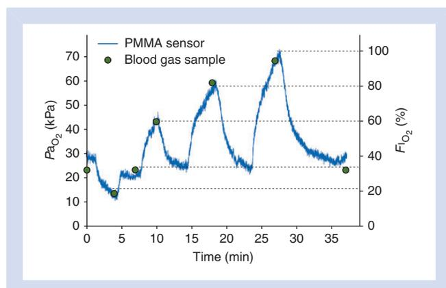
**Fig 1** Arterial  $P_{aO_2}$  responses to  $F_{IO_2}$  step changes in one anaesthetized animal (pig) are plotted against time (sampling rate=10 Hz). The blue line shows  $P_{aO_2}$  recorded by the PMMA sensor, the circles show results from arterial blood gas sampling at 0, 4, 7, 10, 18, 27, and 37 minutes;  $F_{IO_2}$  at these time points was 21, 35, 60, 80, 100, and 35% respectively. The dotted horizontal lines highlight the  $F_{IO_2}$  values at the time when blood samples were taken.
